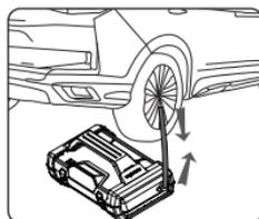
4.1 The inflatable hose is connected to the output port of the air inflator, and then tighten the nut, and the other end is connected to the car tire;
