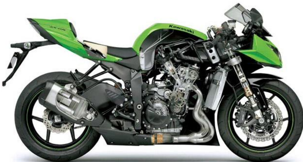
Figure 2) – Kawasaki Ninja 300R Cross Section (Motogokil. 2014)
